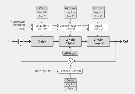
Basically, a comb filter is a delay with a feedback path. Incoming signals pass the delay section and a certain amount of the signal is then being fed back into the input. The signals making their rounds in this feedback loop generate a tone that can be controlled by various parameters to achieve specific sonic characteristics and a dedicated pitch – the comb filter is turned into a resonator / sound source.
