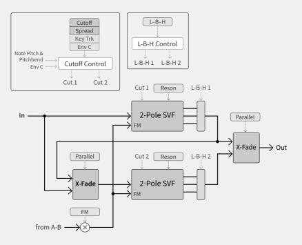
The spacing between both cutoff-points is variable ("Spread"). The filter characteristics can be swept continuously from low through band to high-pass mode ("L–B–H"). Both filters work in series by default but can be continuously shifted to parallel operation ("Parallel").
